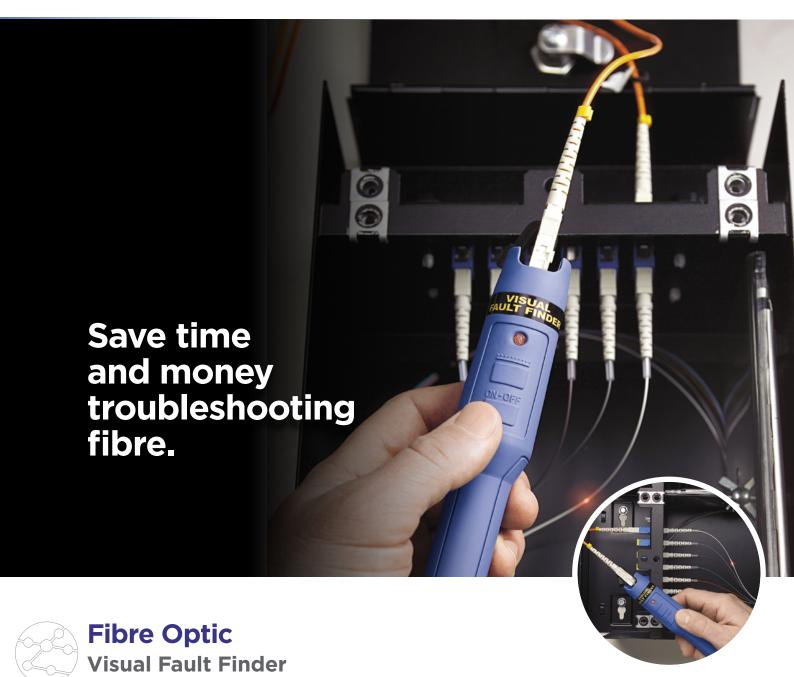
The Visual Fault Finder is a light source used to locate breaks, poor mechanical splices and damaged connectors in fibre optic cables.
