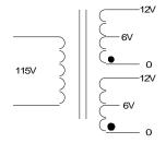
\* Secondaries windings are designed to be connected in series or parallel. Windings are not intended to be used independently.
