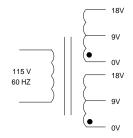
\* Secondary windings are designed to be connected in series or parallel. Windings are not intended to be used independently.
