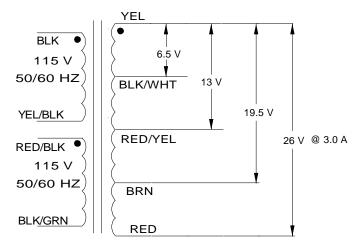
**Technical note:** Primary windings are designed to be connected in series or parallel.
