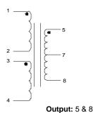
Input (115V): Input 1 & 2 Connect 1&3, 2&4 Input (230V): Input 1 & 4 Connect 2&3
