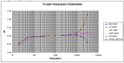
\* 600:600Ω, 10K:10KΩ, 100K:100KΩ, 1M:1MΩ, and other impedances (secondaries can all be used at ¼ value when placed in parallel) are optional as long as input voltage is ≤4.2Vrms and current is ≤7mA.
