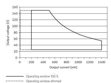
Make sure that the LED driver is operated within the given window under all operating conditions. Special attention needs to be paid at dimming as the forward voltage of the connected LED modules varies with the dimming level, due to the implemented amplitude dimming technology. Coming below the specified minimum output voltage of the LED driver may cause the device to shut-down.
