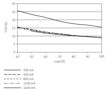
100 % load corresponds to the max. output power (full load) according to the table on page 3.
