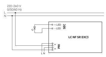
Device with loop through wiring function.
