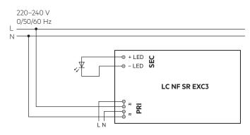
Device with loop through wiring function.
