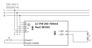
Device with loop through wiring function.
