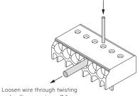
and pulling or using a Ø 1mm release tool
