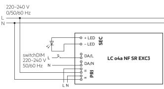
Device with loop through wiring function.
