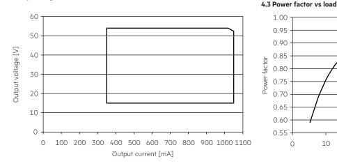
Make sure that the LED driver is operated within the given window under all operating conditions. Coming below the specified minimum output voltage of the LED driver may cause the device to shut-down.
