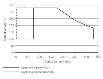
Make sure that the LED driver is operated within the given window under all operating conditions. Special attention needs to be paid at dimming and DC emergency operation as the forward voltage of the connected LED modules varies with the dimming level, due to the implemented amplitude dimming technology. Coming below the specified minimum output voltage of the LED driver may cause the device to shut-down. See chapter "6.9 DC operation" for more information.
