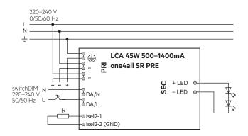
Device with loop through wiring function.
