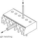
Loosen wire through twisting and pulling or using a  $\emptyset$  1 mm release tool
