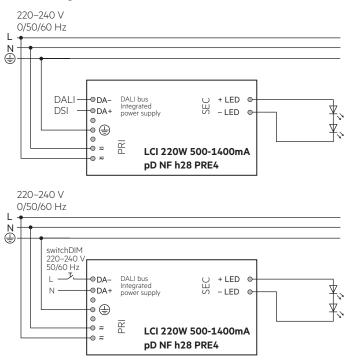
DALI bus power supply has to be deactivated when using switchDIM or corridorFUNCTION. Otherwise it could be damaged.
