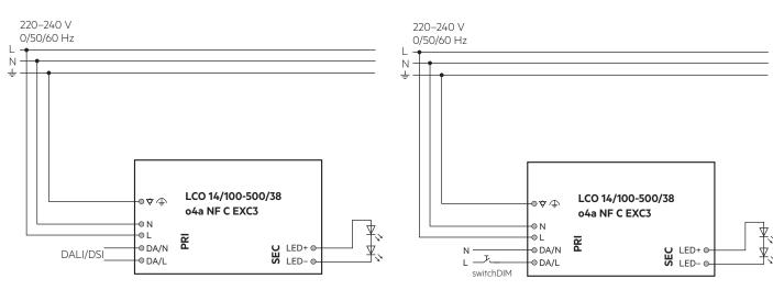
For wiring in dimming operation with ready2mains refer to the ready2mains Gateway data sheet.
