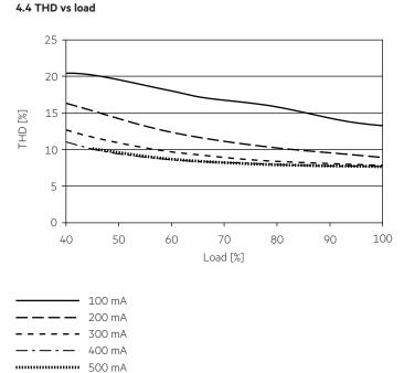
100 % load corresponds to the max. output power (full load) according to the table on page 3.
