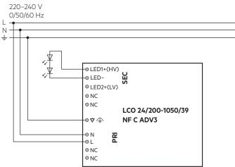
For wiring in dimming operation with ready2mains refer to the ready2mains Gateway data sheet.
