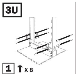
Reverse the mounting ears and secure them as shown using screws provided with your UPS/battery pack.
