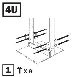
Reverse the mounting ears and secure them as shown using screws provided with your UPS/battery pack.
