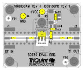
For optimal OIP3 performance, the ground plane to the left and right side around the backside paddle of the WJA1021 should be removed as shown in the above PCB layout.
