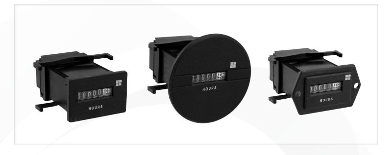
The Redington Model 711 provides a family of compact 7 figure, AC Hour Meters. Models are available in the standard industry housings, 2- Hole rectangular, flush-round and flush-rectangular. A choice of two rectangular panel cutouts are offered 1.45" X 0.95" [36.8mm X 24.1mm] or 1.45" X 0.87" [36.8mm X 2.1mm]. The Round meter has a panel cutout of 1.99" [50.5mm].
