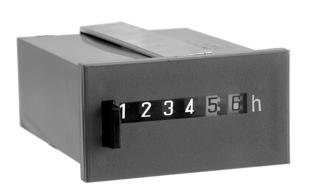
A rectangular style AC hour meter designed to complement existing meters in control panels. Available in 6 figure reset or 7 figure non-reset. The nonreset model incorporates a retaining clip to lock into panel, while the reset version has a metal bracket and screw.
