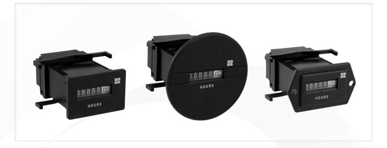
The Redington Model 711 provides a family of compact 7 figure, AC Hour Meters. Models are available in the standard industry housings, 2- Hole rectangular, flush-round and flush-rectangular. A choice of two rectangular panel cutouts are offered 1.45" X 0.95" [36.8mm X 24.1mm] or 1.45" X 0.87" [36.8mm X 2.1mm]. The Round meter has a panel cutout of 1.99" [50.5mm].
