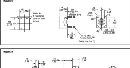
Terminal Pins (3) Solderable  $.017 \pm .003$  $0.432 \pm 0.076$  Dia.
