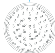
24-61 Service rating 1 61 Contact, Size 24
