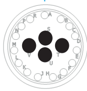
16-19* Service rating 1 15 Contacts, Size 20 4 Contacts, Size 16
