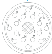
16-CX Service rating 1 17 Contacts, Size 20 1 Co-Axial Contact, for RG316/U
