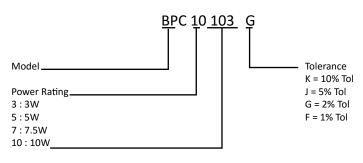
Resistance Code Tolerance  $0.1~\Omega:0R100$   $10~K\Omega:103$  First two digits significant, last digit: number of trailing zeros
