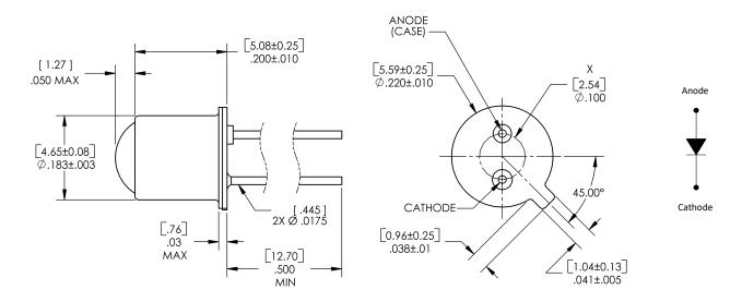
X THIS DIMENSION CONTROLLED AT HOUSING SURFACE.
