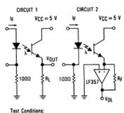
Light source is pulsed LED with  $t_f$  and  $t_f \leq 500$  ns. IF is adjusted for VOUT = 1 Volt.
