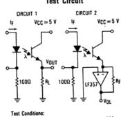
Light source is pulsed LED with  $t_f$  and  $t_f \leq 500~\text{ns.}$  IF is adjusted for VOUT = 1 Volt.
