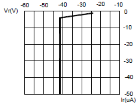
Reverse Current vs Reverse Voltage
