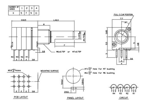
P08xS - POTENTIOMETER WITH ROTARY SWITCH MODULE
