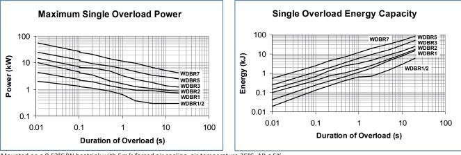
Mounted on a 0.53°C/W heatsink with 5m/s forced air cooling, air temperature  $25^{\circ}$ C.  $\Delta R \le 5\%$ .
