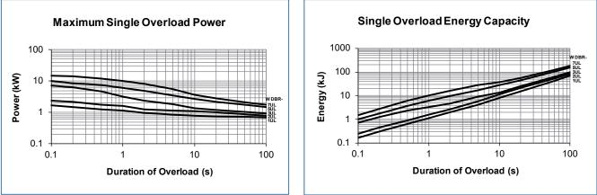
Mounted on a 0.53°C/W heatsink with 5m/s forced air cooling, air temperature 25°C.  $\Delta R \leq 5\%$ .
