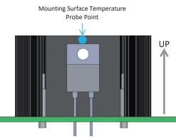
These data relate to a normal application condition with fins obstructed by a PCB and non-ducted airflow, and may be used for practical thermal design.
