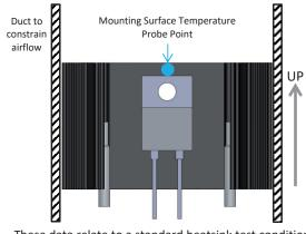
These data relate to a standard heatsink test condition with unobstructed fins and ducted airflow, and are included for comparison purposes.
