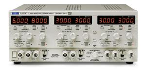
The **PL303QMT** triple has one output of 0-6V at 0-8A with 1mV and 1mA resolution. The other two outputs are each 0-30V at 0-3A with quad-mode switching providing tracking operation or true parallel to give 0-30V at 0-6A from a single output. All outputs are linear regulated.
