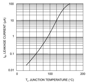
Fig. 3 Leakage Current vs Junction Temperature
