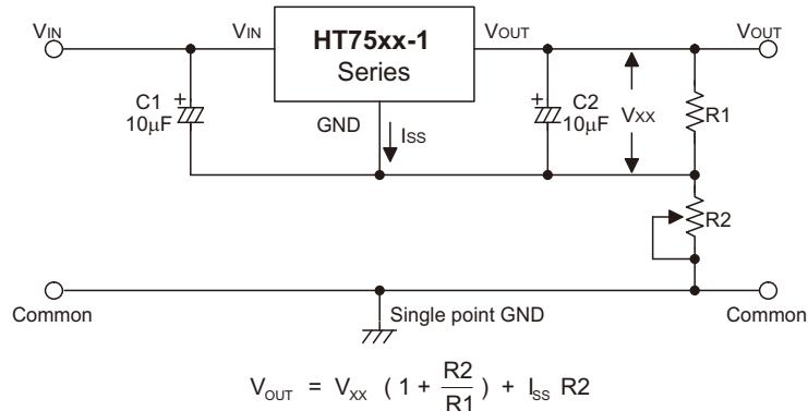
**Circuit for Increasing Output Voltage**
