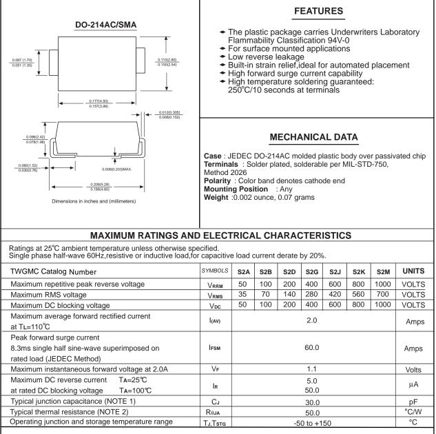
Note: 1. Measured at 1MHz and applied reverse voltage of 4.0V D.C.
