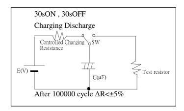
Where Y: Multiple of momentary rated power of test resistor However,a converted value shall not exceed 750 V in any case.
