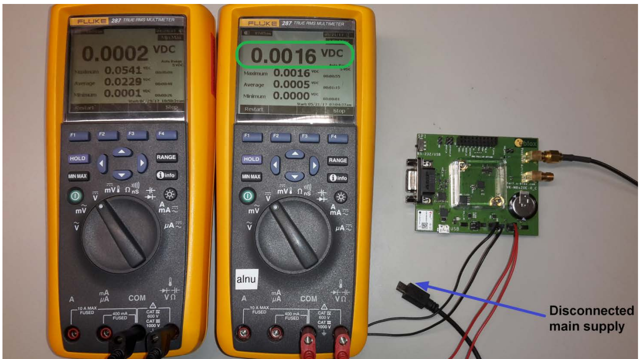
Figure 10: Setup to measure the V_BCKP current consumption of ZOE-M8B on EVK-M8BZOE
