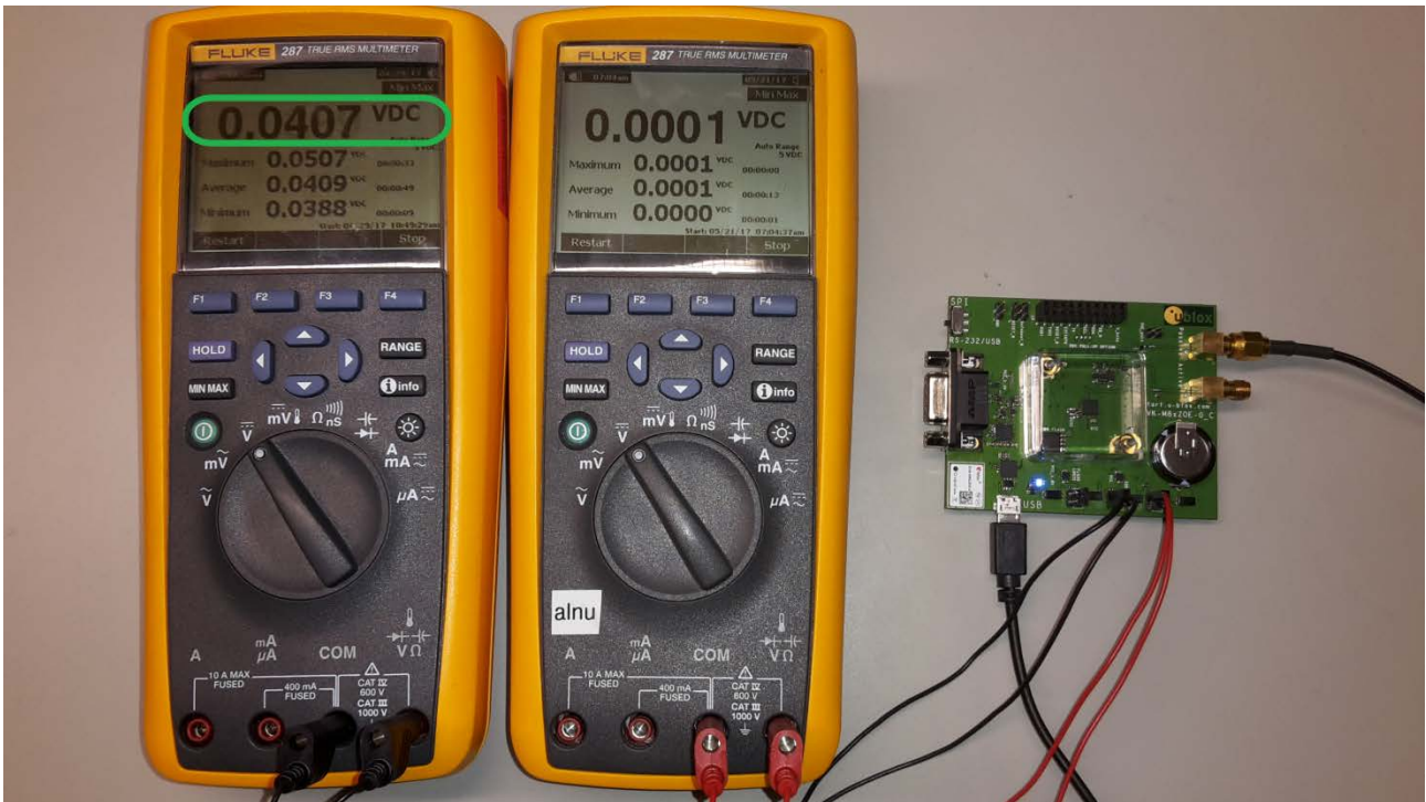
Figure 9: Setup to measure the VCC current consumption of ZOE-M8B on EVK-M8BZOE
