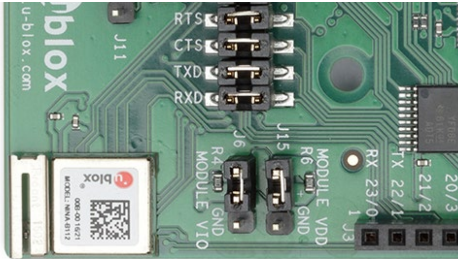
Figure 9: Placement of R4 and R6 (10 \Omega resistors)
