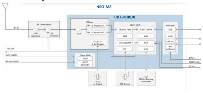
Figure 1: NEO-M8 block diagram
