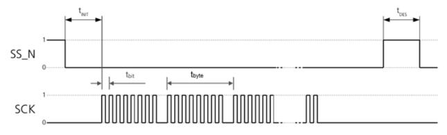
Figure 3: SPI timing diagram
