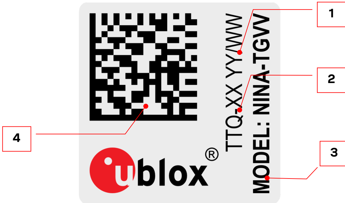
Figure 16: Location of product type number on the NINA-B1 series module label
