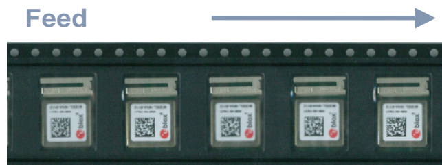
Figure 13: Orientation of NINA-B112 modules on tape
