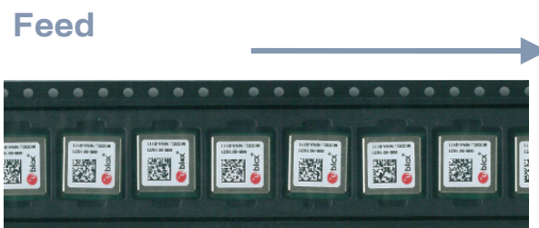
Figure 12: Orientation of NINA-B111 modules on tape
