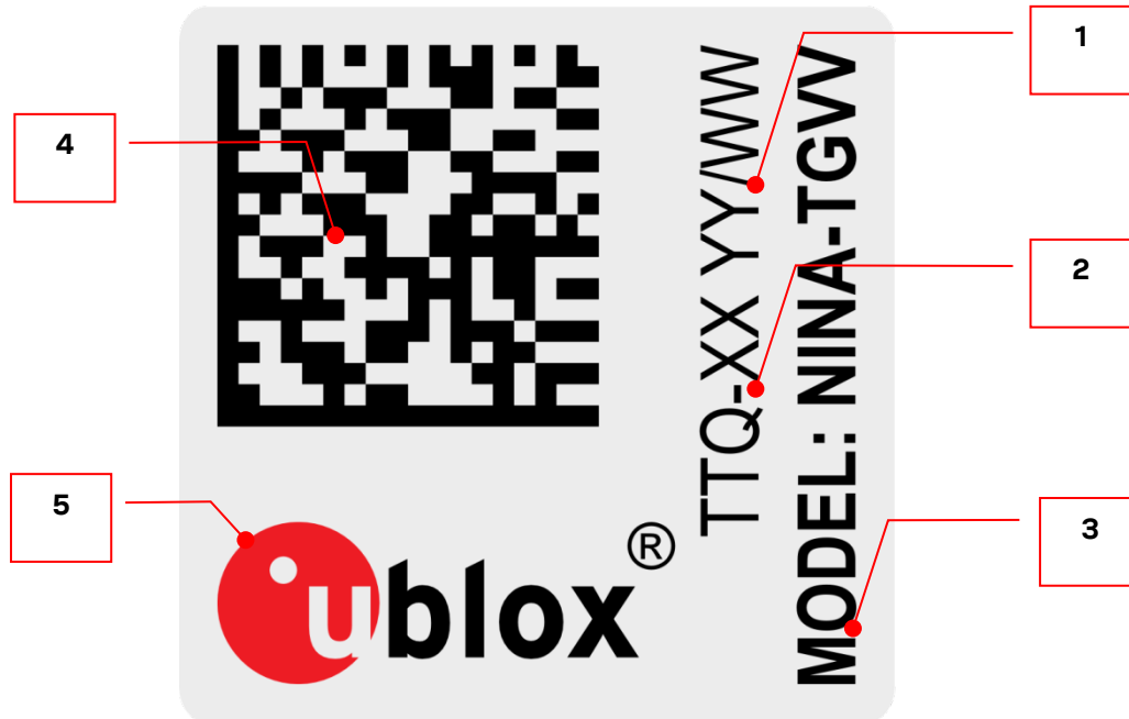
Figure 13: Layout of the NINA-B50 module label
