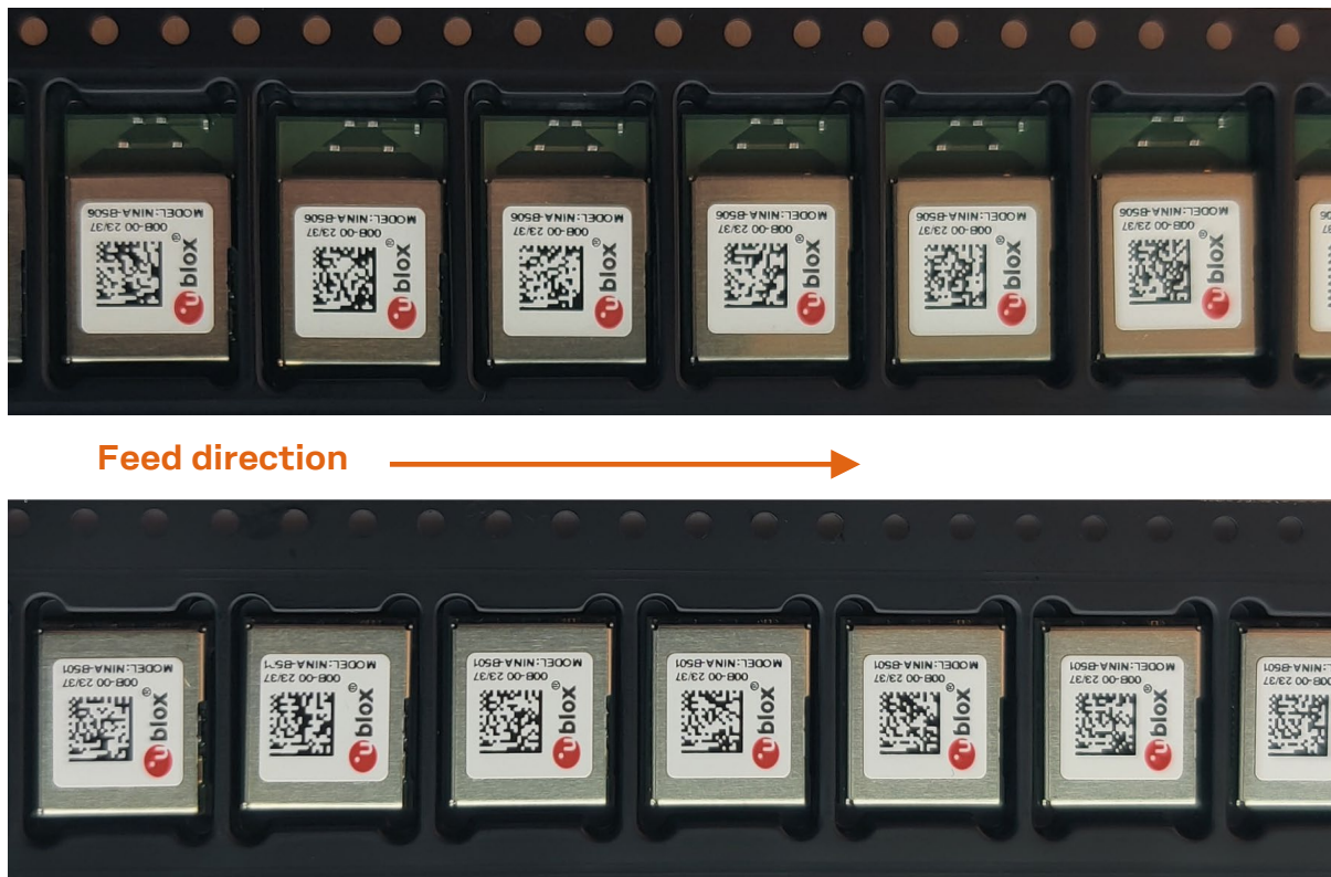
Figure 10: Orientation of NINA-B50 modules on tape
