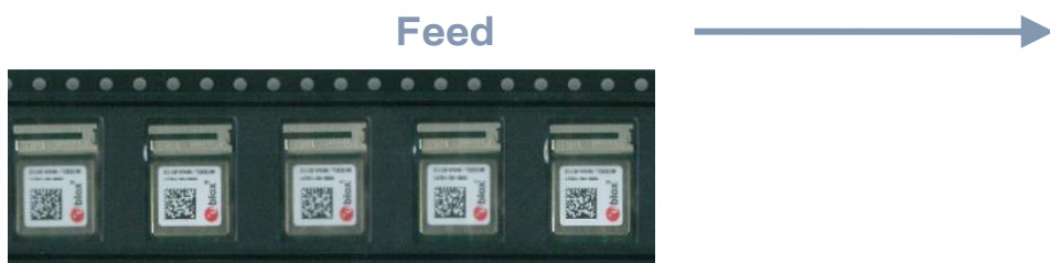
Figure 13: Orientation of NINA-W152/NINA-W156 module on tape
