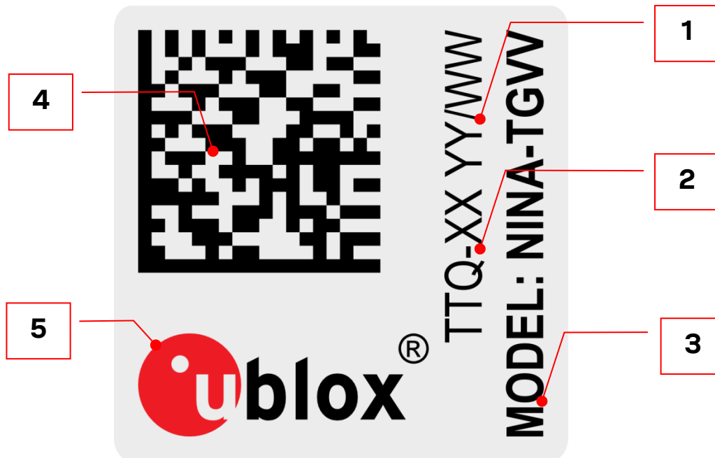
Figure 16: Location of product type number on the NINA-W15 series module label
