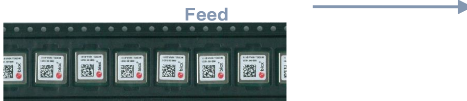
Figure 12: Orientation of NINA-W151 module on tape
