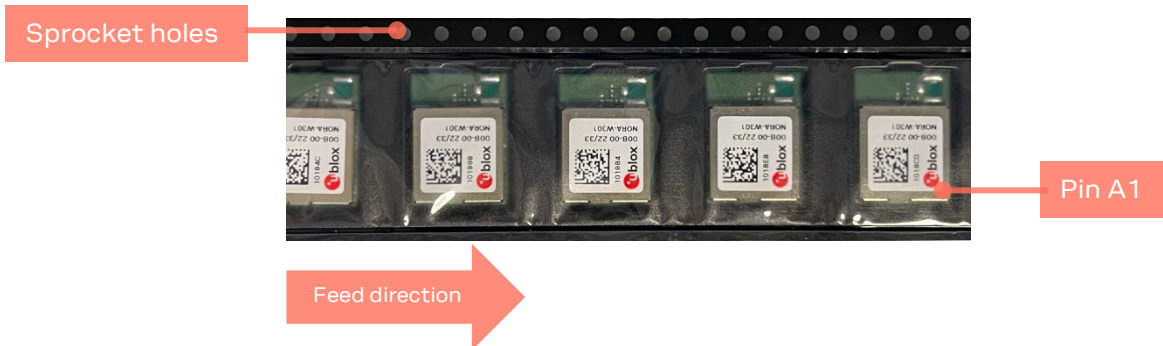
Figure 6: NORA-W301 module on tape orientation
