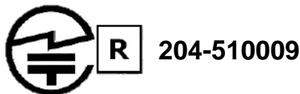
Figure 7: Giteki mark, R and the ODIN-W2 MIC certification number. The "Indoor use only" information translated into Japanese below is mandatory if the product is operating in the 5.2/5.3 GHz band.
