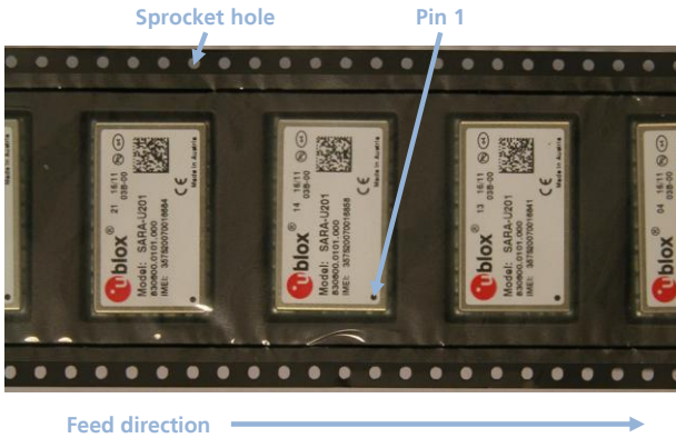
Figure 16: Orientation for SARA-U2 series modules on tape
