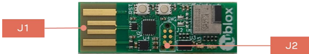
Figure 3: Available connectors, pinout, and designators
