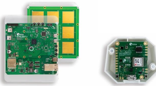
Figure 1: Complete XPLR-AOA-3 kit - showing the EVB-ANT-1 application board (front left), ANT-B10 antenna board (back left) and C209 tag (right)
