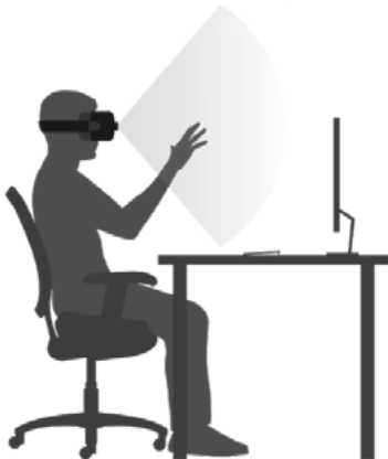
The Leap Motion Controller features a 140x120° field of view and an interactive tracking range of up to 60cm (24") or more.
